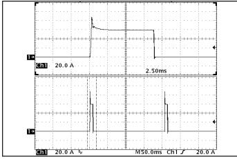
Figure 15: Load current (20A/div) as a function of time when the converter attempts to turn on into a 1 m $\Omega$  short circuit. Top trace (2.5ms/div) is an expansion of the on-time portion of the bottom trace.
