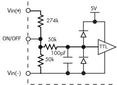
Figure B: Internal ON/OFF pin circuitry
