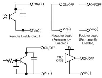
Open Collector Enable Circuit Direct Logic Drive *Figure A: Various circuits for driving the ON/OFF pin.*
