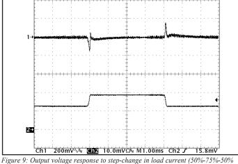
Figure 9: Output voltage response to step-change in load current (50%-75%-50% of lout(max);  $dI/dt = 0.1A/\mu s$ ). Load cap:  $15\mu F$ ,  $450m\Omega$  ESR tantalum cap and  $1\mu F$  ceramic cap. Top trace: Vout (200mv/div), Bottom Trace: Iout (20A/div).
