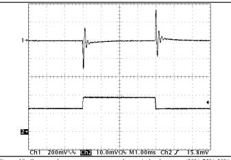
Figure 10: Output voltage response to step-change in load current (50%-75%-50% of lout(max):  $dI/dt = 5A/\mu s$ ). Load cap:  $470\mu F$ ,  $15m\Omega$  ESR tantalum cap and  $1\mu F$  ceramic cap. Top trace: Vout (200mv/div), Bottom Trace:lout (20A/div).
