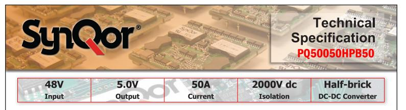
The PQ50050HPB50 PowerQor<sup>®</sup> Peta Half-brick converter is a next-generation, board-mountable, isolated, fixed switching frequency DC-DC converter that uses synchronous rectification to achieve extremely high conversion efficiency. The Peta series converters offers industry leading outputcurrent for standard "half-brick" module. RoHS Compliant (see last page).
